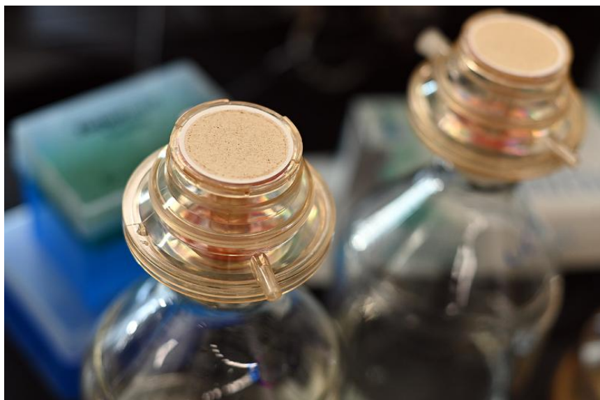
Water samples are pulled through filters, leaving behind organic material to analyze.
